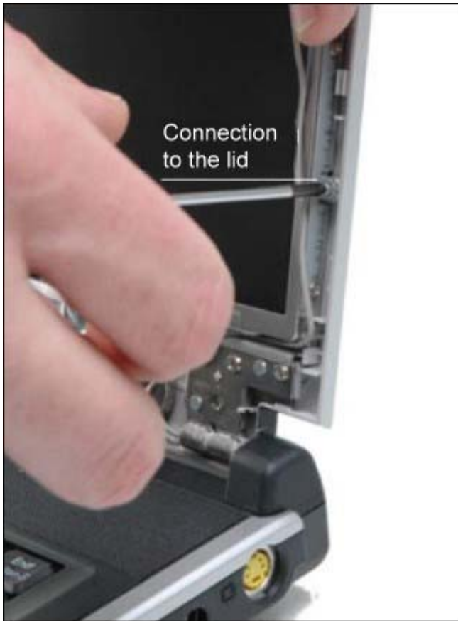
Remove the screws between holding frame and laptop lid in order to get to the holding screws of the LCD
