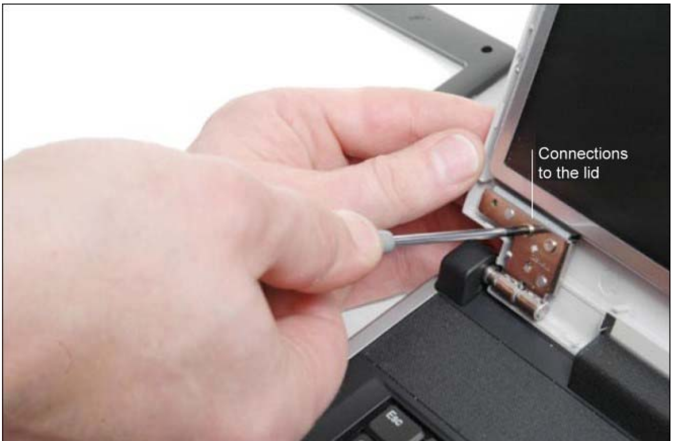
Remove the screws between holding frame and laptop lid in order to get to the holding screws of the LCD
